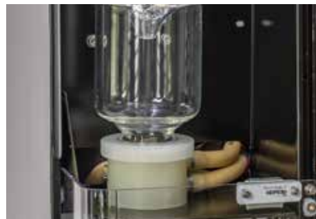
PROTECTION WITH BLACKLINE AS WELL AS PTFE COATING AROUND SENSITIVE PARTS. POLYPROPYLENE SPLASHHEAD OPTIONAL.
